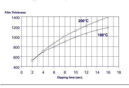
Film thickness ( $\mu$ m) vs. dipping time (sec) and preheating temperature (°C) - Araldite KU 600-1 applied to 1.5 mm tin plate
