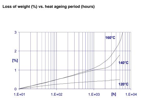
These curves were obtained by testing Araldite KU 600-1 powder applied to iron plate (1.5x70x150 mm) and cured for 1 hour at 180°C; film thickness approx. 750 um. They indicate by extrapolation that, if the permissible loss of weight is to be 2% over 25'000 hours, the maximum service temperature of the coating is 135°C. Similarly, if the loss of weight may be 10% (VDE 0368), the maximum service temperature would be 160°C.
